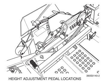
Figure 4-8. Height Adjust Pedal Locations
